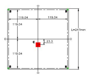
s – standoff's platform of PCB antenna Ø 7.5 mm
